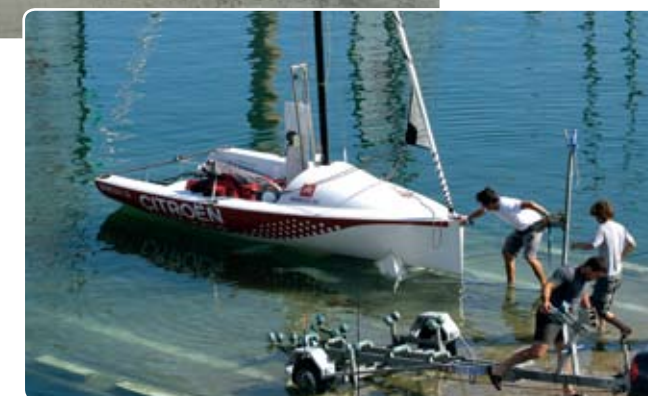
LEFT The boat features a high aspect square top main and generous jib.
